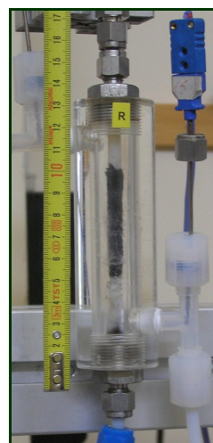
Fig. 3. Catalytic reactor for \text{NaBH}_4 hydrolysis
