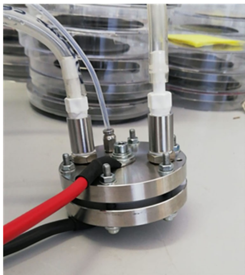
FIGURE 3 Electrolysis cell for the characterization of electrodes
